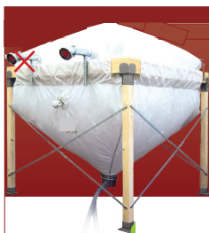
3.6 ton capacity Flexi-Bulk silo with posts and beams (not included). Specify auger or vacuum for transport from silo to boiler. Optional single fill connection at bin requires bringing fill hose to bin (as shown). Fill connection can also be made to home exterior.
